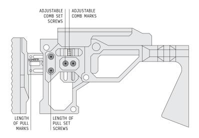
The butt-stock of your MPR $^{m}$  Rimfire rifle folds away to the right side of the rifle capturing the bolt and stowing in the folded position via our Magnelock $^{m}$  technology. Simply depress the butt-stock release button on the left side of the stock frame and fold the butt-stock to the right.
